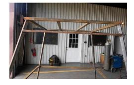
Make sure you weld the 24-inch piece to where the 72-inch piece is in the middle of it. This is the bottom step for your ladder.
