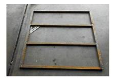
• Weld the pieces together using the welder.
